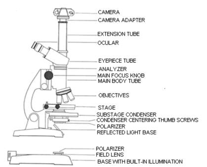
You can find the names of the parts of the microscope from the diagram below:
